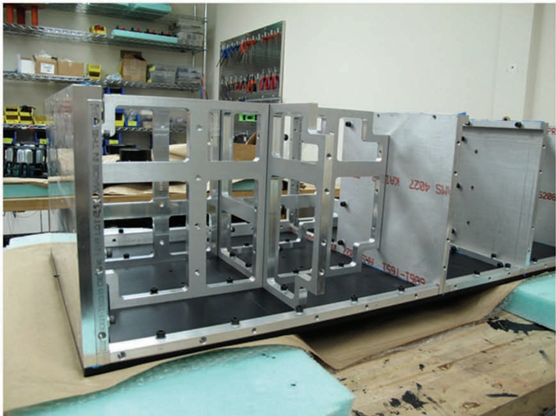
At Magico's Berkeley Facility the Q5 Subchassis Are Assembled from the Machined Structural Parts
